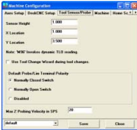
After the X and Y axis motion is complete, the Z-axis is moved down toward the sensor to record the tool length. The tool setter must be positioned in the specified X-Y position before the M96 command is issued.
