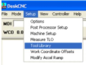
Click on the desired tool length and type in the measured length.
