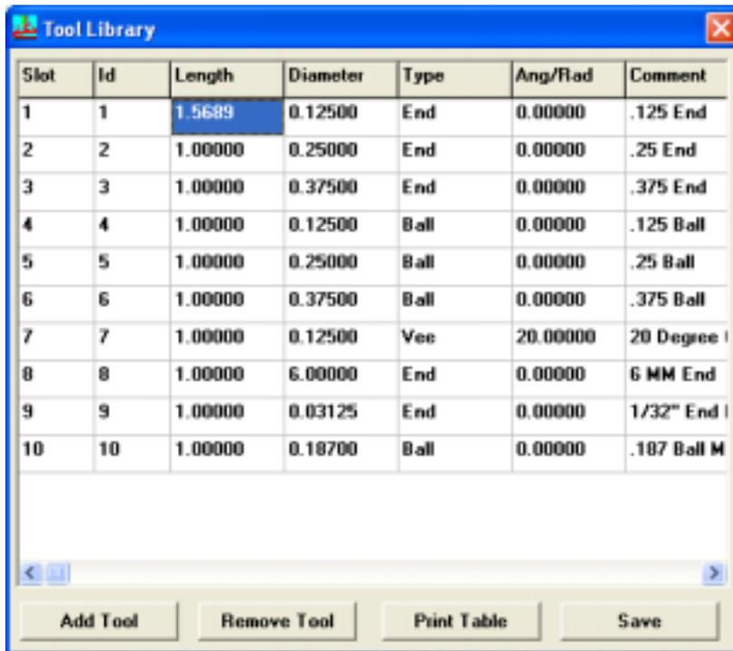
A screenshot of the 'Tool Library' dialog box. It contains a table with 7 columns: Slot, Id, Length, Diameter, Type, Ang/Rad, and Comment. The 'Length' column is highlighted. Below the table are buttons for 'Add Tool', 'Remove Tool', 'Print Table', and 'Save'.
